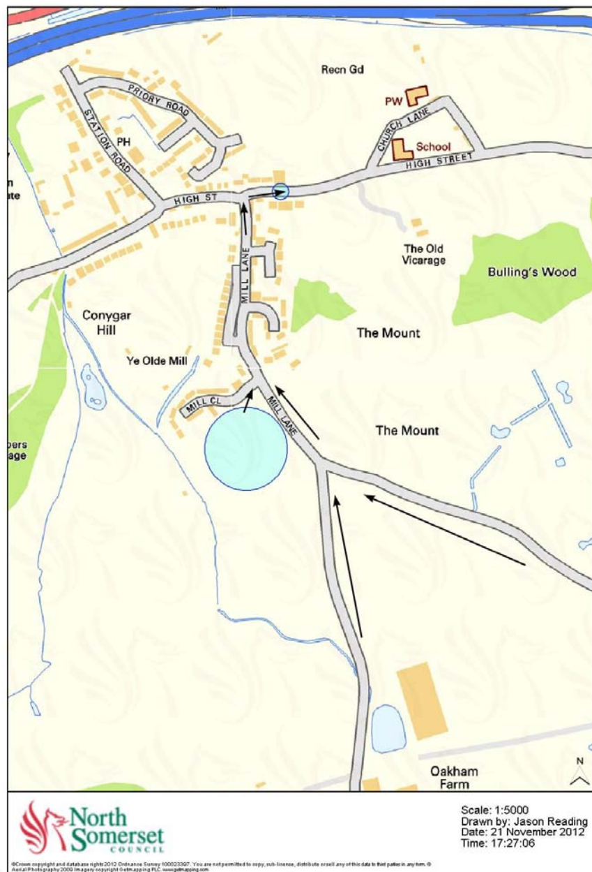
Figure 29: Location of pooling water and the conveyance route
